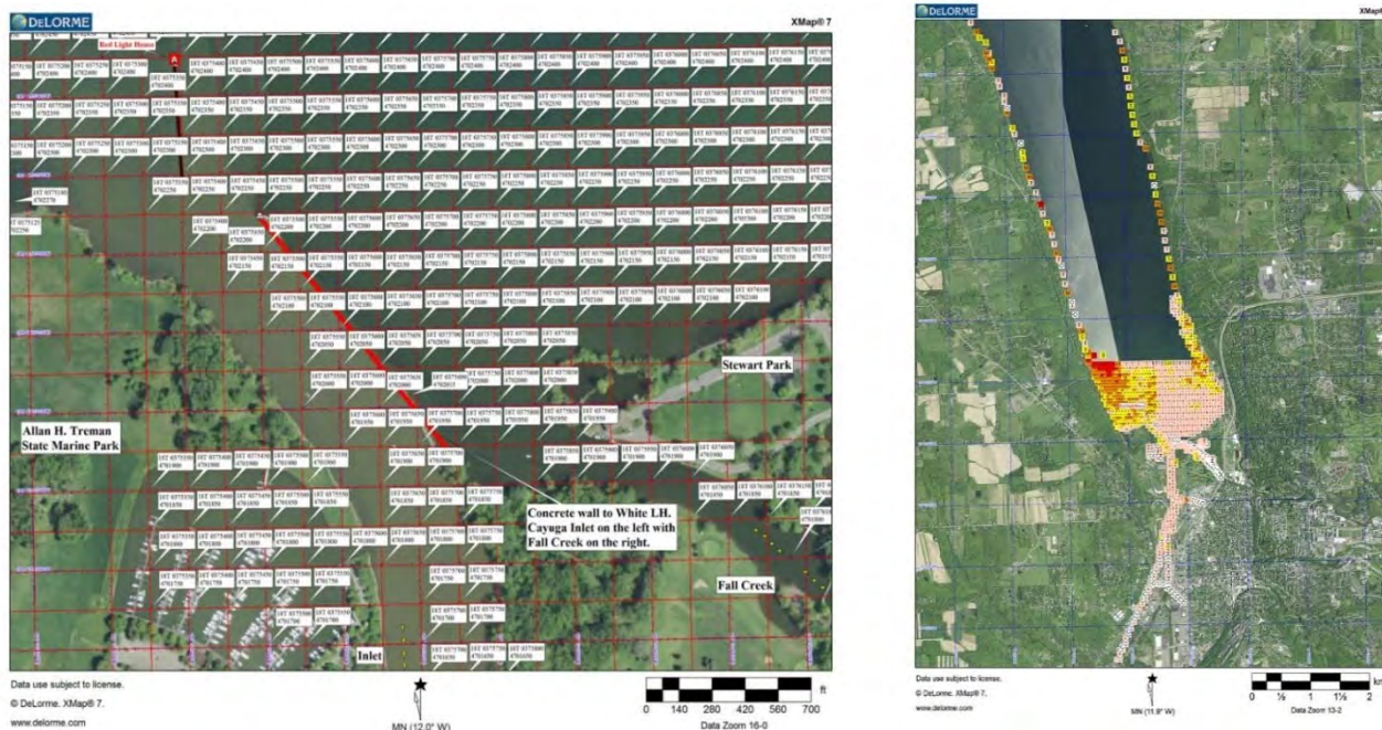
Figure 15. Example of a small section of our UTM grid used to predetermine locations to sample aquatic plant presence and abundance. Locations sampled are at points defined by the line intercepts of the NAD 1983 X coordinate East and NAD 1983 Y coordinate North. We have used this grid method of determining sample locations since 2012 on this project. The pictorial on the left shows the total area searched in 2018 and the estimated density for All Species Combined at each rake-toss location.
